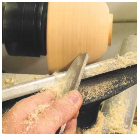
▲ Pic.4 The face of the bowl can be cleaned up in the more traditional way, with the tool flat on the toolrest. The scraper's worst enemy is vibration, so keep the rest close to the work where possible
